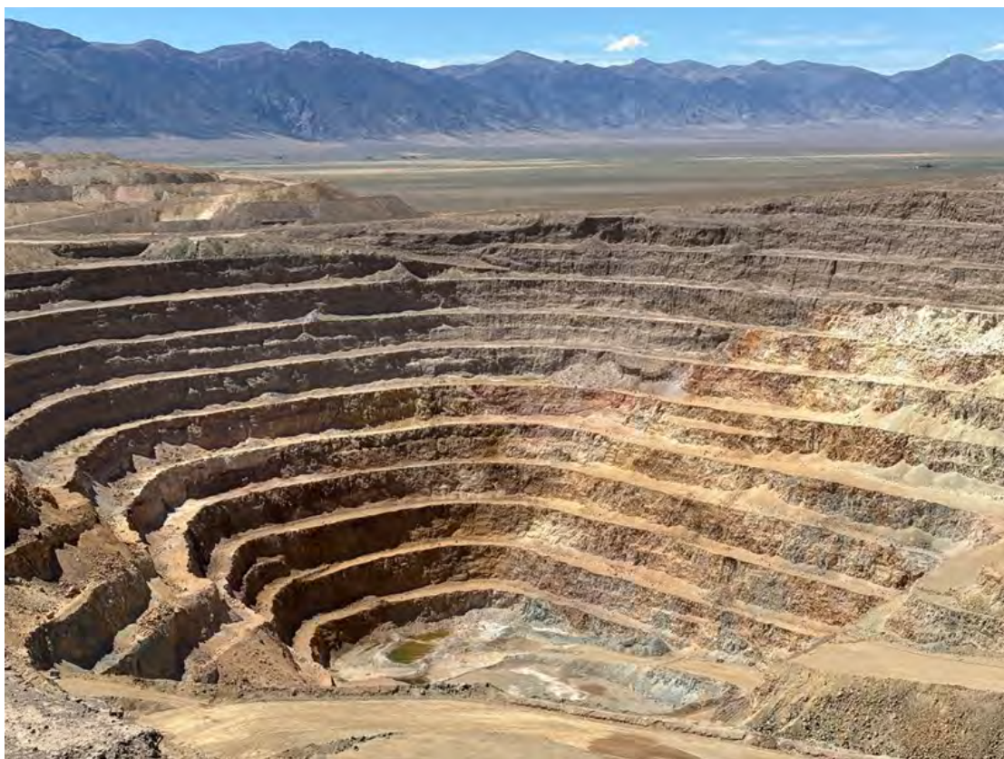
View looking northwest at west and north walls of Gold Hill pit with Toiyabe Range in the background. Note the post-mineral basin-range fault that drops valley-fill gravels (grey rock) against altered tuff of Mt. Jefferson near right-middle of frame. This is the fault that truncated east-west striking veins mined underground during the 1930s. Bench heights are about 35 feet.
