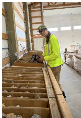
Performing pXRF analysis on historic drill core for Sun Silver, 2025.
