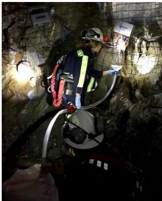
Sampling an underground seep for geochemical characterization influent water. My client (in the foreground) called the sample collection device a modified beer bong.
