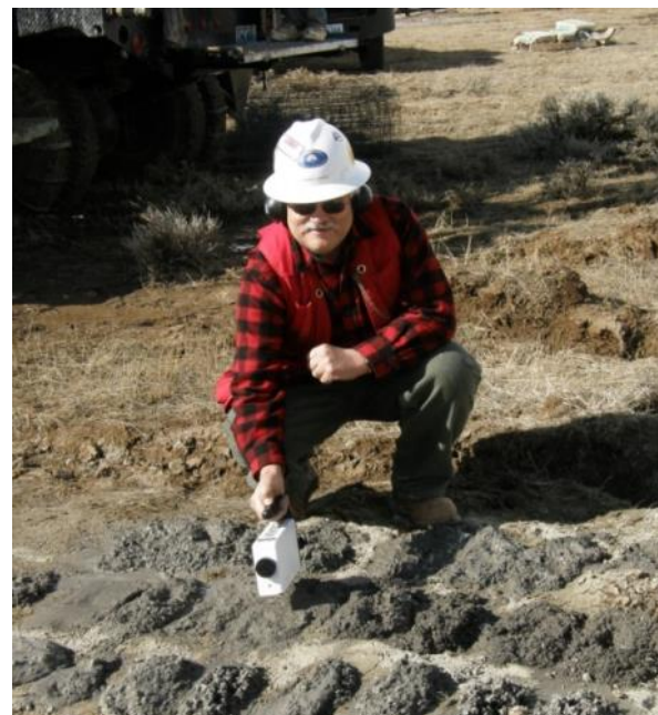
Looking for uranium—scanning rotary mud drill cuttings with scintillometer, Powder River Basin, WY, March 2010.
