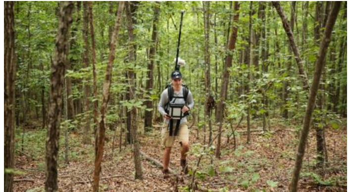
Me in North Carolina running a backpack magnetometer
